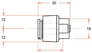
Pipe Insertion Depth: 23mm
